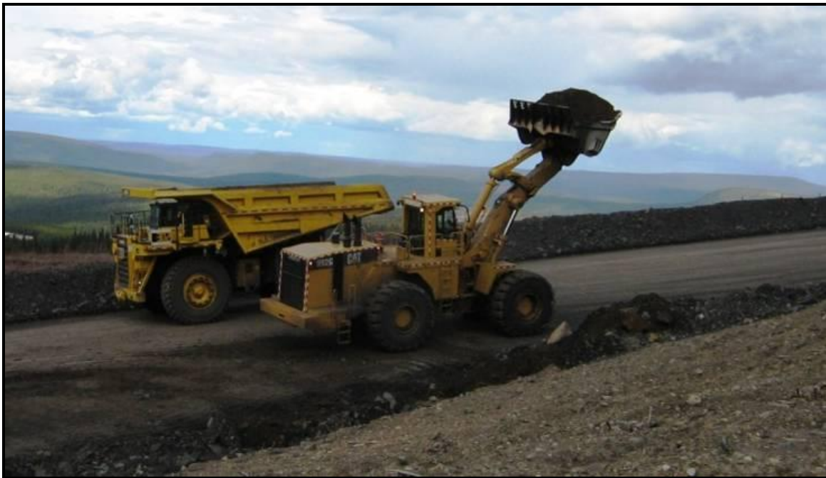
Truck operator positions truck so that he can back in keeping the loader on his good (left) side.
