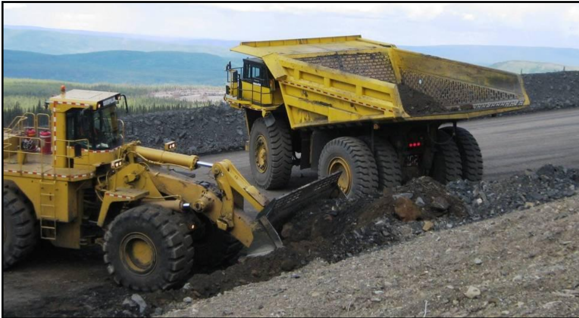
Truck operator waits in truck cab while loader fills the truck bed.
